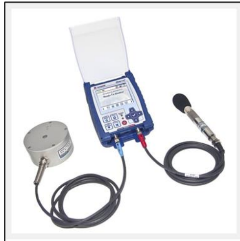
Figure 6 — An example of the equipment (InstanTel Micromate) that can be used to measure vibrations. InstanTel Micromate can be connected to both the geophone and the microphone to measure both ground and air vibrations
