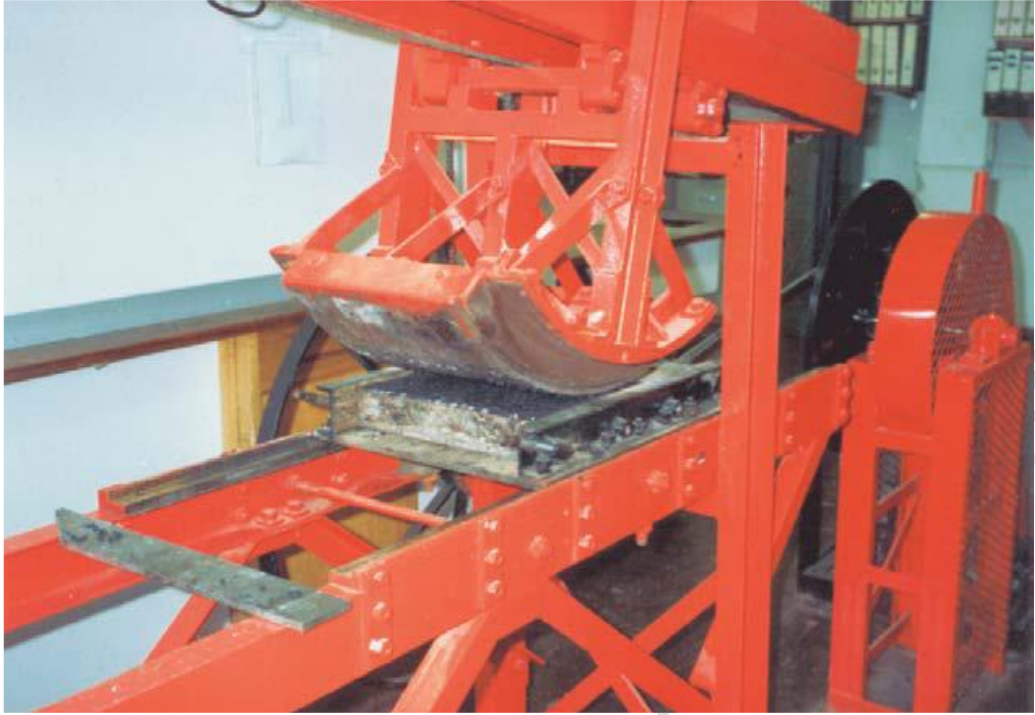
Figure C.2 — Compaction of Slab for Wheel Tracking Test
