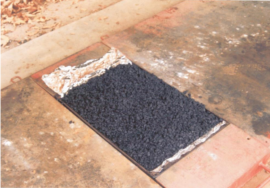
Figure C.6 — Compacted Sample using Rolling Wheel Compaction
