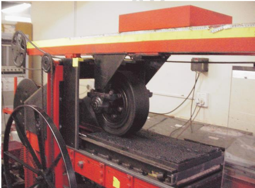
Figure C.2 — Compaction of Slab for Wheel Tracking Test
