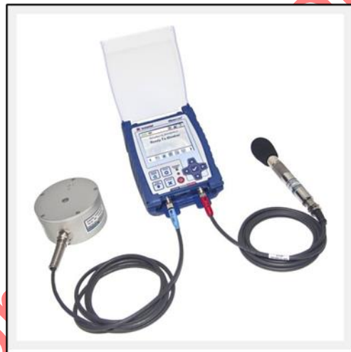
Figure 4 — An example of the equipment (Instantel Micromate) that can be used to measure vibrations. Instantel Micromate can be connected to both the geophone and the microphone to measure both ground and air vibrations
