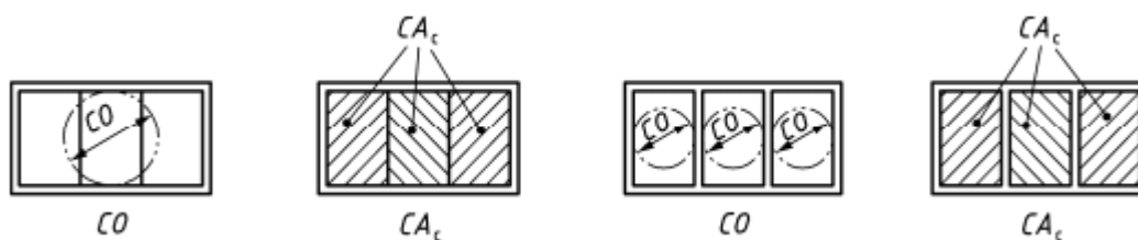
Figure E.4 — Examples of determination of Clear Areas of multiple covers/gratings
