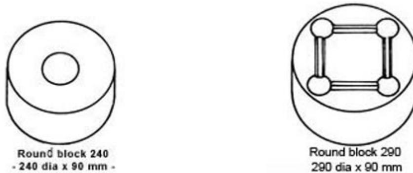
Figure 10 — Circular-type blocks used for building composite column
