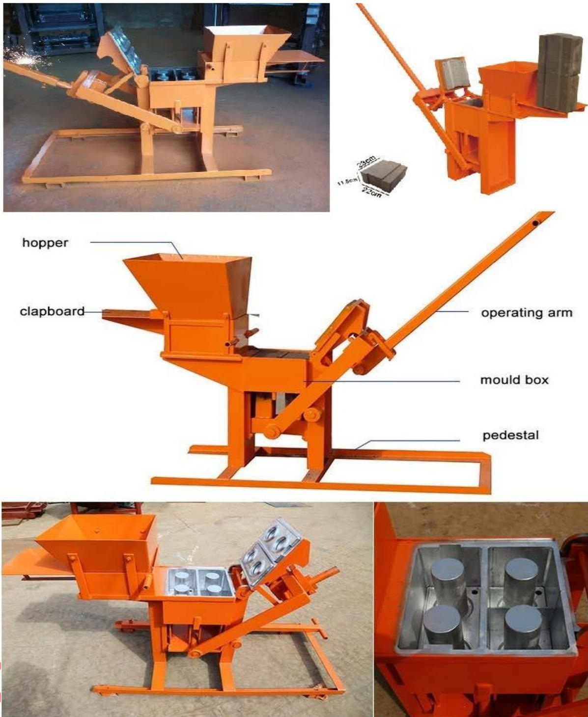
Figure 15 — Interlocking compressive block making manual hand machine
