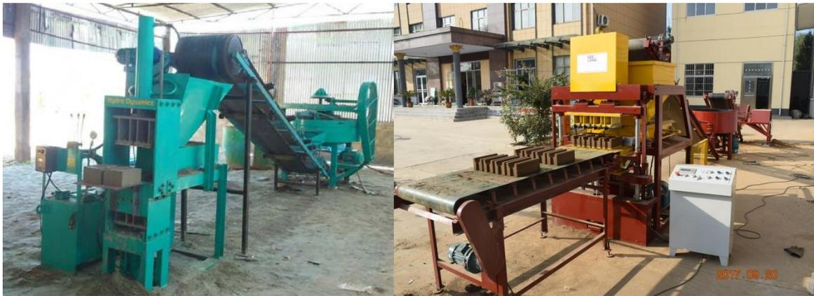
**Figure 18** — Interlocking compressive block making fixed machine.
