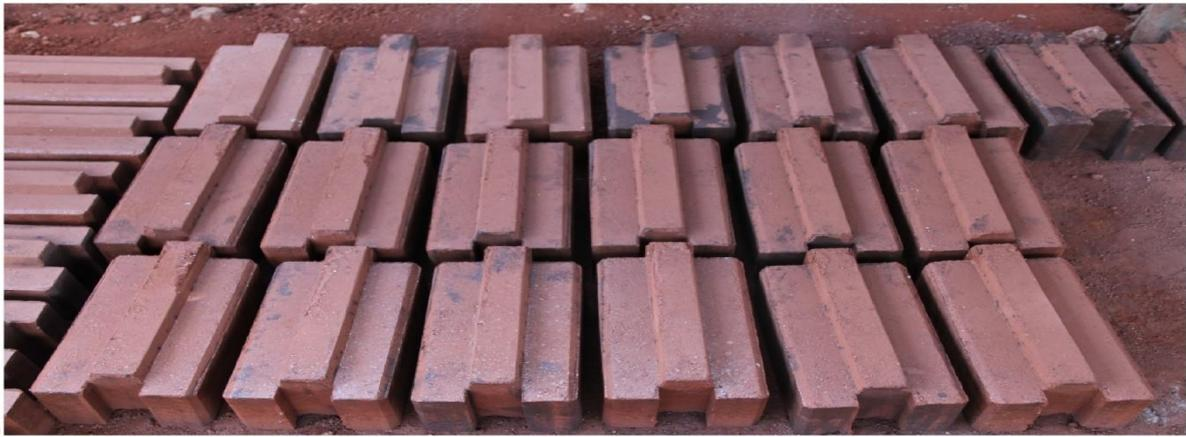
Figure 5 — The African interlock for compressed stabilised earth block
