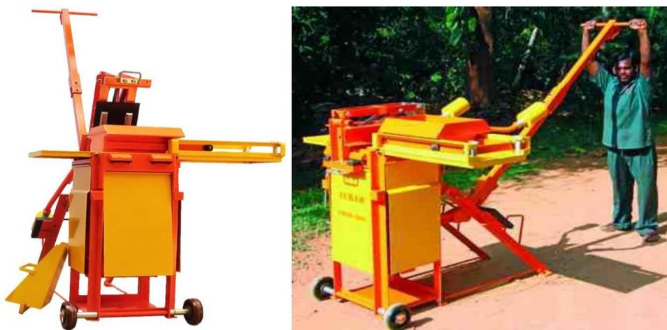
Figure 14 — Auram Press 3000 manual compressed brick making machine
