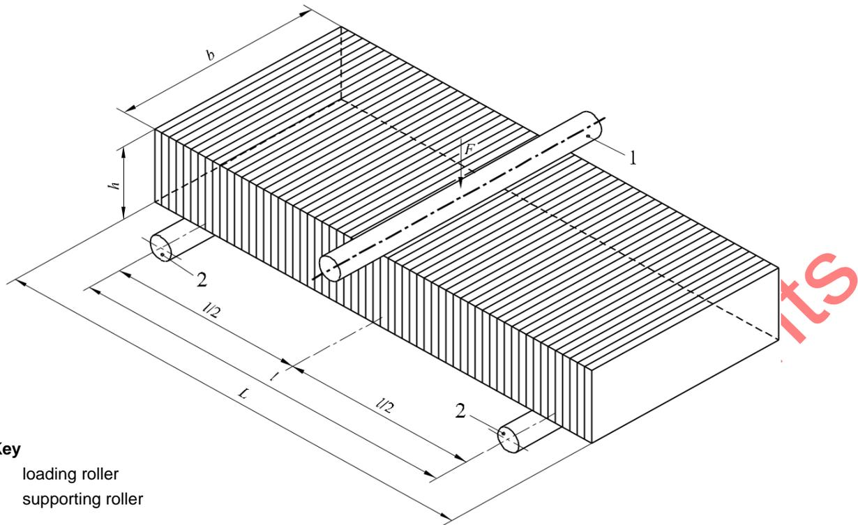
Figure 3 — Test arrangement for a specimen with the load applied parallel to the planes of anisotropy
