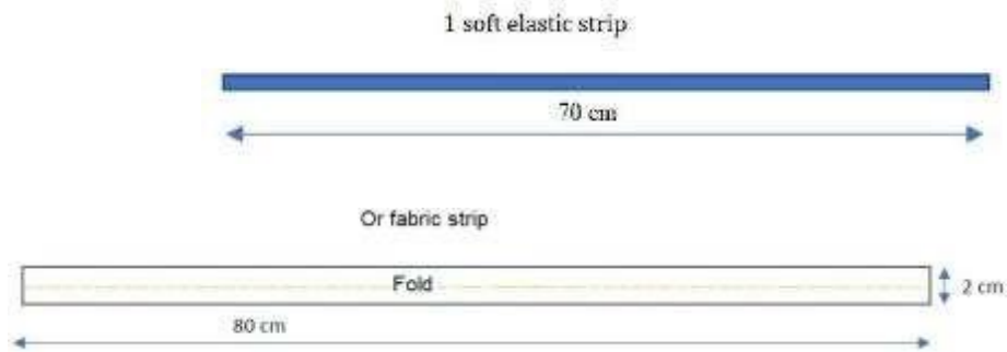
Figure A.2 — Duckbill - Sizing of head harness
