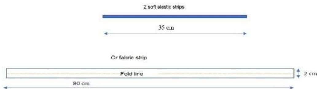
Figure A.5 — Flat-fold - Sizing of the head harness
