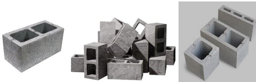
**2.5 Cellular block** is a blocks which contain one or more formed voids which do not fully penetrate the block
