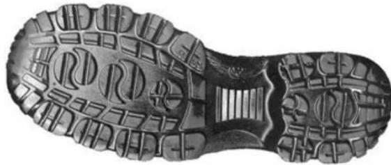
Figure B.2 — Profiled sole of test shoe
