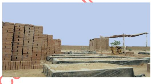
Figure 12 — Brick curing
