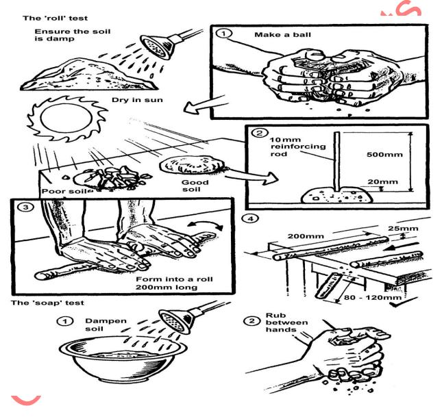
Figure A.1: The 'Roll' and 'Soap' Tests
