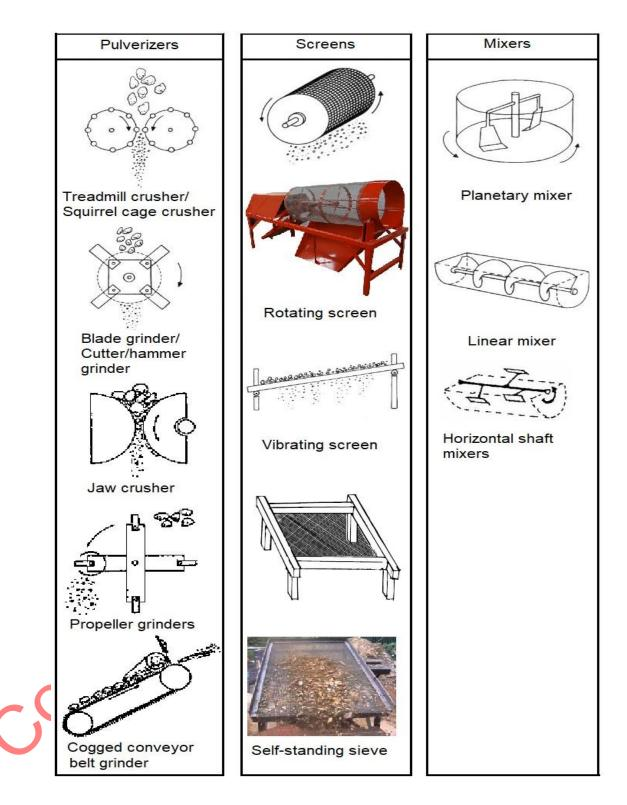
Figure 13 — Pulverisers, screens and mixers for soil preparation
